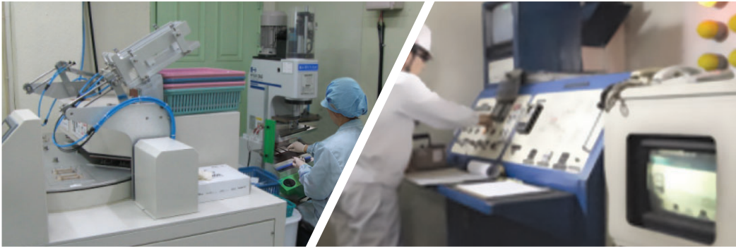
Sanitarily packed products at Class 10,000 clean room are sterilized by gamma-ray using radiation isotope.
