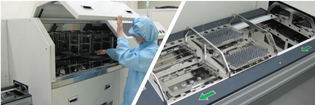
Cleansing process by ultrasonic wave using the 3 rd still distilled, vacuum dry and heating dry sterilization enable ultimately sterilized products and no residues are left on products.
